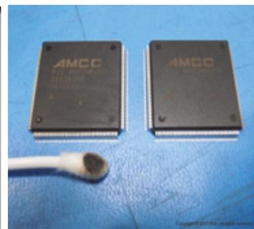
Figure 10. Ghost markings are visible on part 2 (circled)
